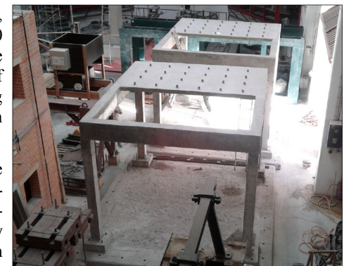
Figure 2: General view of reinforced concrete frames tested on a shake table for Blind Test Challenge.
