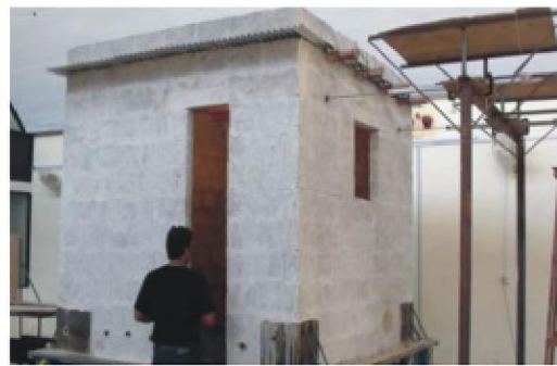
Fig 2. Unreinforced masonry structure with instrumentations attached
