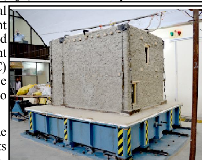
Figure 8: Shaking Table Test of Hunza House
