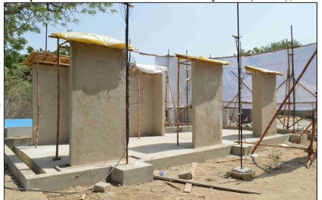
Figure 9: Rain testing of wall panels
