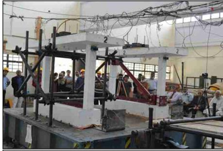
Figure 1: Dynamic Test Setup of BRB Strengthened RC Frame
