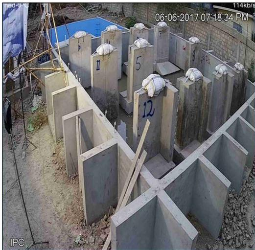
Figure 8: View of flood testing facility with specimen walls
