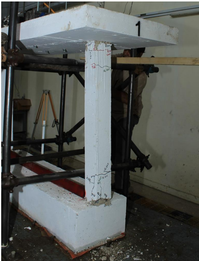
Fig. 13 Damage zones in column of control frame
