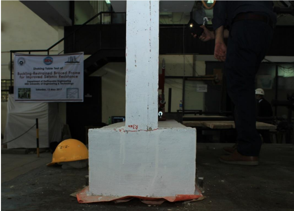
Fig. 12 Crack at the column-base beam junction in BRB strengthened frame
