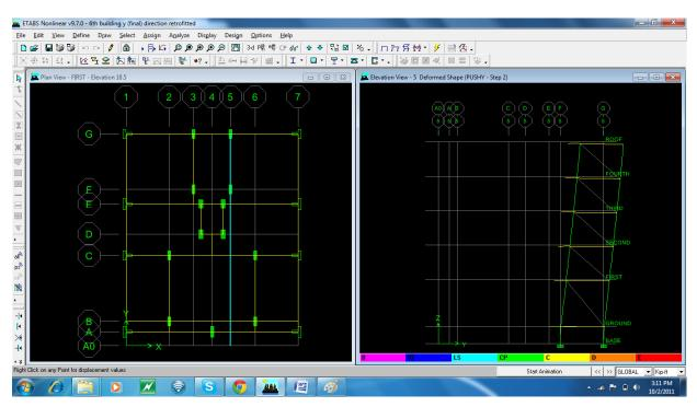
Mechanism or Deformed shapes at Performance Point for grid-5
