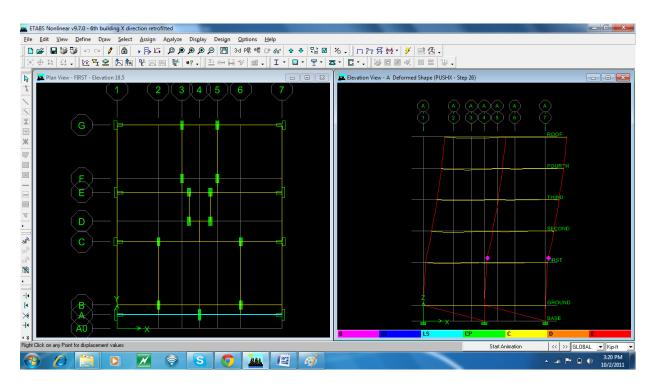
Mechanism or Deformed shapes at Performance Point for grid-A
