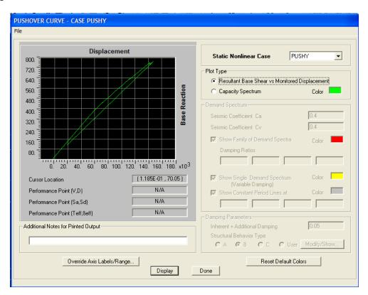
Figure 6. Pushover curve for Y-direction
