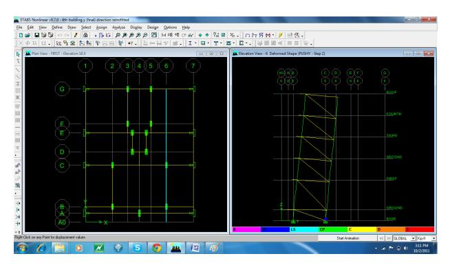
Mechanism or Deformed shapes at Performance Point for grid-6
