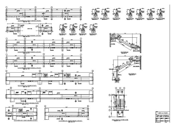
Figure 4. Structural beam elevations and sections for typical floor plan and staircase
