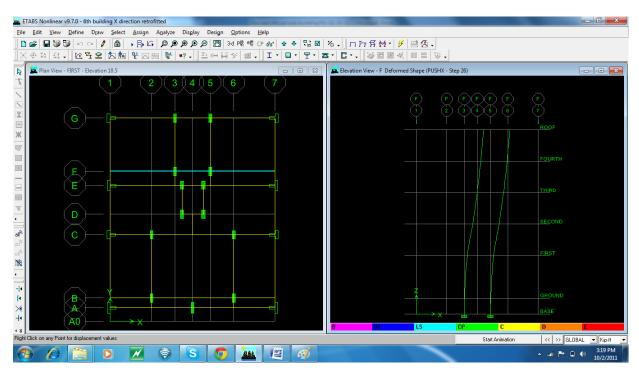
Mechanism or Deformed shapes at Performance Point for grid-F
