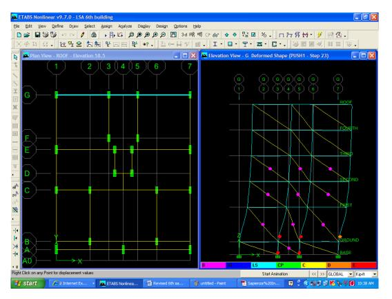
Figure 11. Hinge deformation vs. acceptance criteria for x-direction analysis
