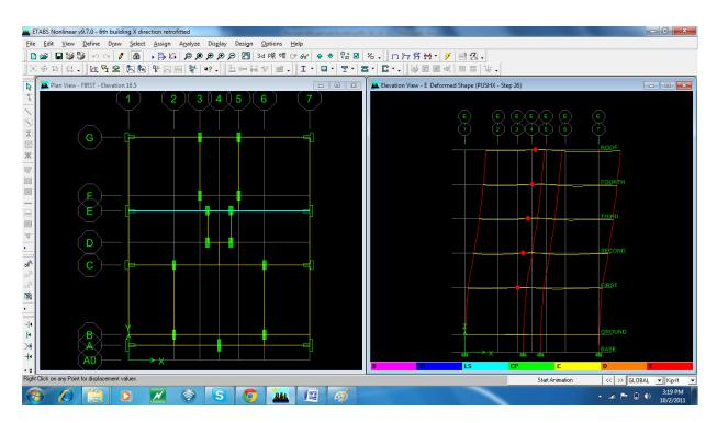
Mechanism or Deformed shapes at Performance Point for grid-E
