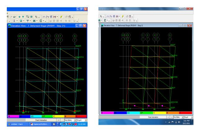
Figure 14. Hinge deformation vs. acceptance criteria in Y-direction before retrofit (left) after retrofit (right)
