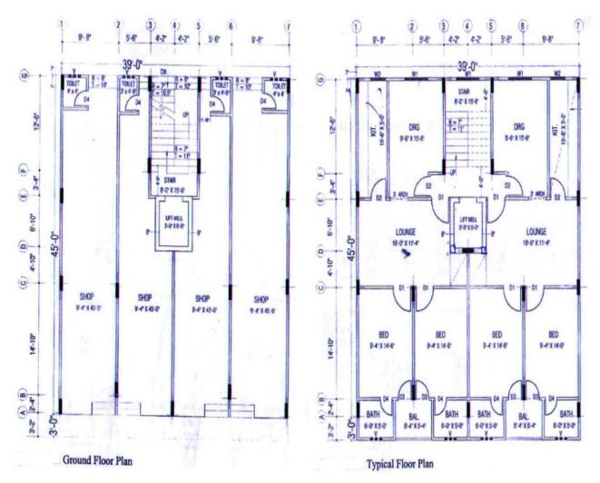
Figure 1. Architectural plan of ground (left) and plan of typical floors (right)
