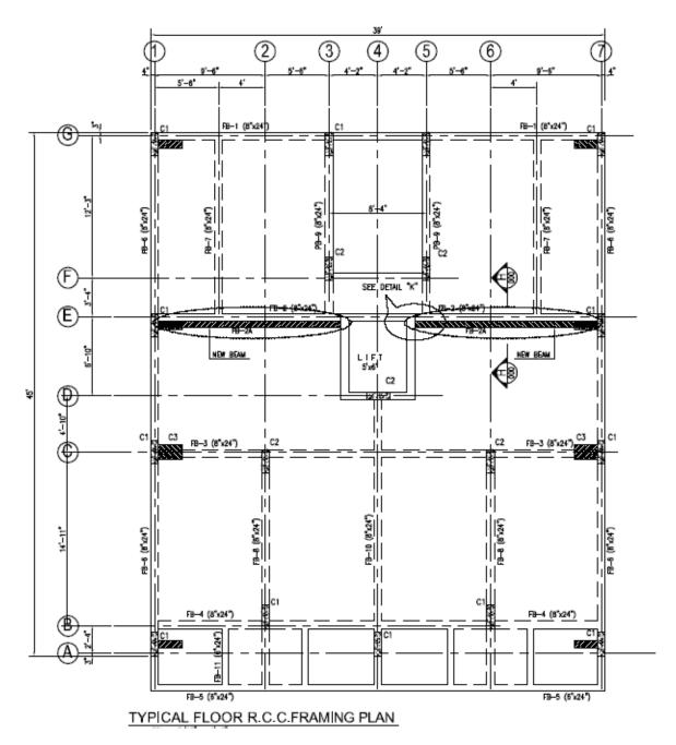
Figure 17. Locations of strengthened beams and columns
