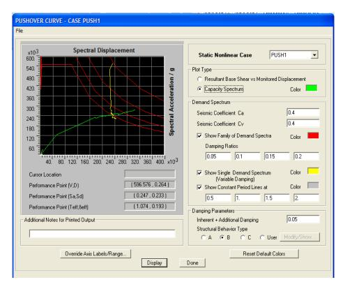
Figure 10. Performance level for X-direction
