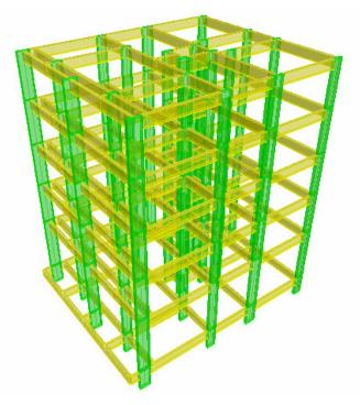
Figure 5. Rendering of linear ETABS model of the building
