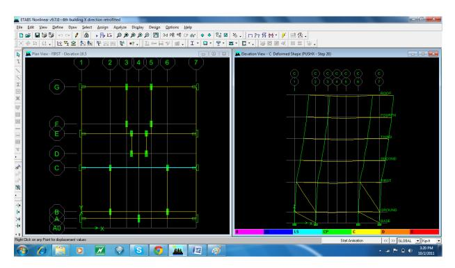
Mechanism or Deformed shapes at Performance Point for grid-C
