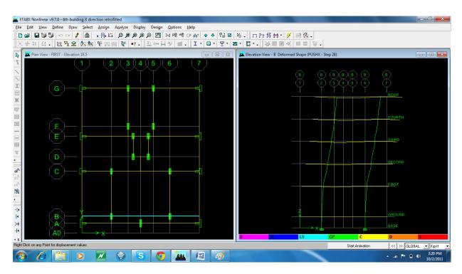
Mechanism or Deformed shapes at Performance Point for grid-B
