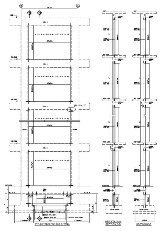
Figure 16. Structural elevation and section of new shear walls
