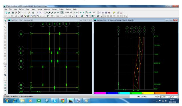
Mechanism or Deformed shapes at Performance Point for grid-D
