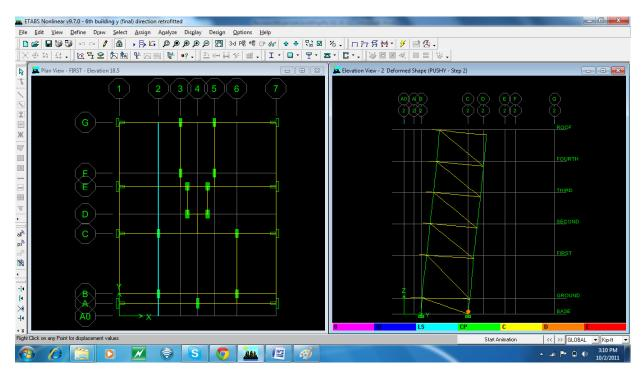
Mechanism or Deformed shapes at Performance Point for grid-2
