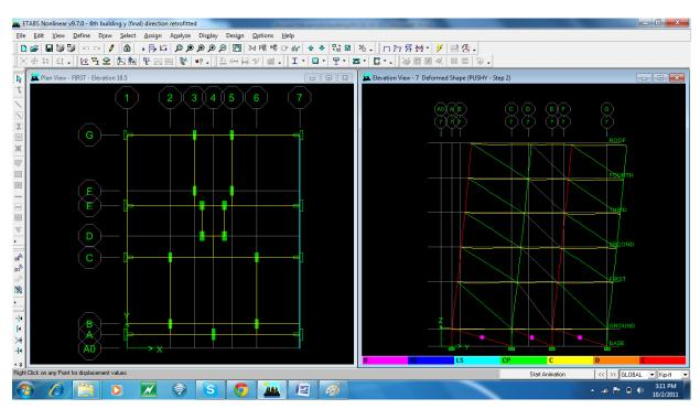
Mechanism or Deformed shapes at Performance Point for grid-7
