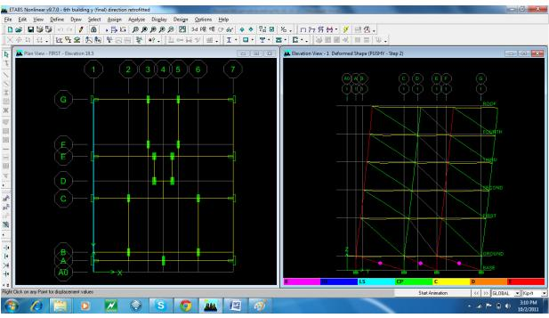
Mechanism or Deformed shapes at Performance Point for grid-1
