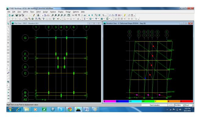
Mechanism or Deformed shapes at Performance Point for grid-G
