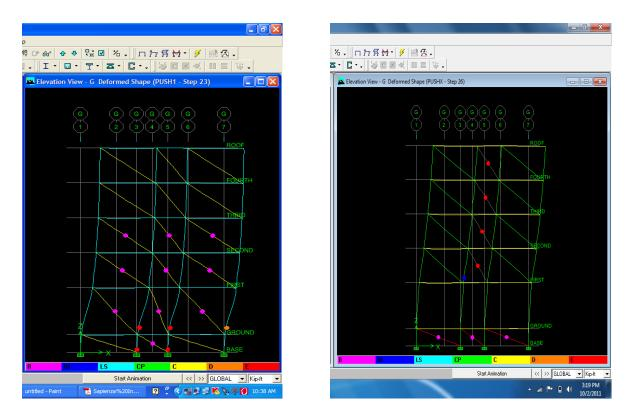
Figure 15. Hinge deformation vs. acceptance criteria in Y-direction before retrofit (left) after retrofit (right)
