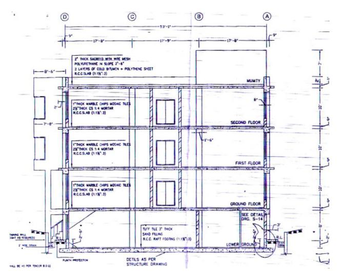
Figure 5. Architectural typical section in elevation
