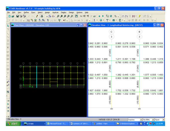
**Required Reinforcement in Beams**
