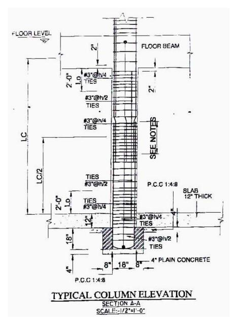
Figure 7. Structural drawings for columns
