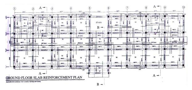
Figure 10. Reinforcement details for floor slabs
