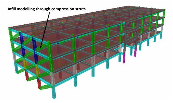
Figure 11. Rendering of linear ETABS model of the building
