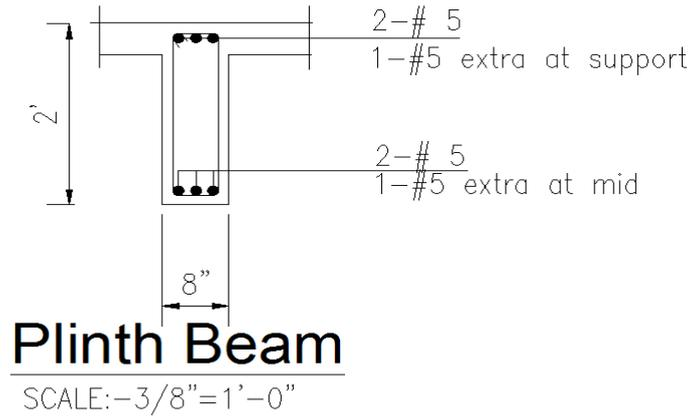
Figure 13. Typical plinth beam section
