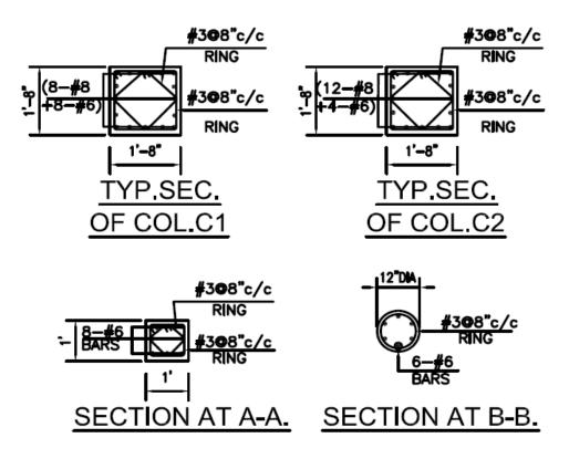
Figure 10. Typical column sections
