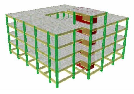
Figure 14. Rendering of linear ETABS model of the building
