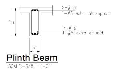
Figure 13. Typical plinth beam section
