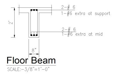
Figure 12. Typical floor beam section
