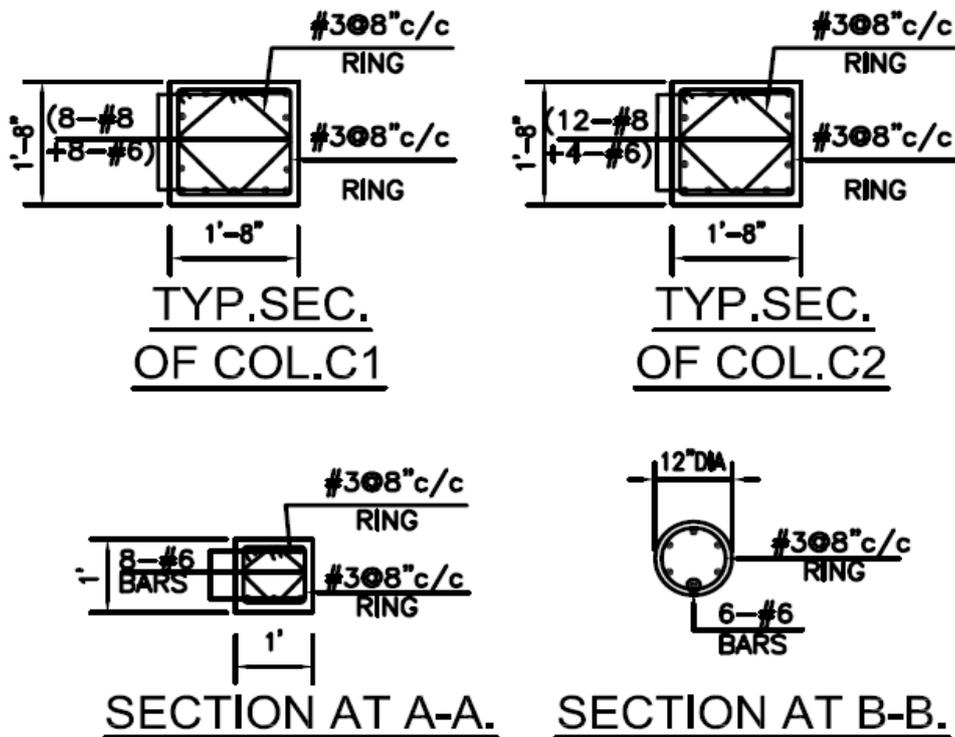
Figure 10. Typical column sections
