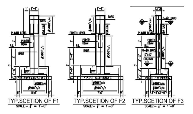
Figure 9. Sections of footings and columns
