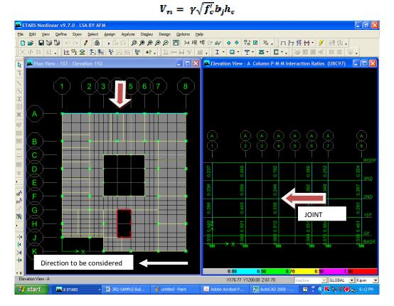
Figure 15. Joint checked for shear by hand calculation
