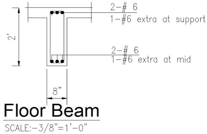
Figure 12. Typical floor beam section
