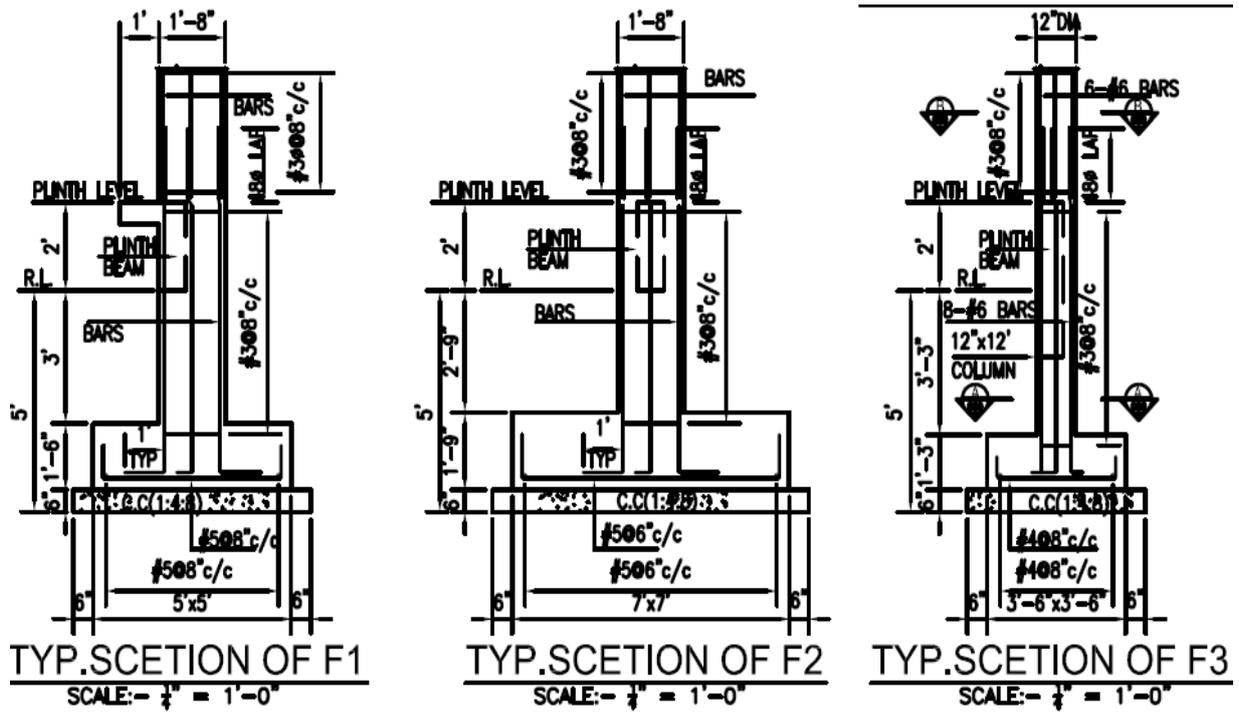
Figure 9. Sections of footings and columns
