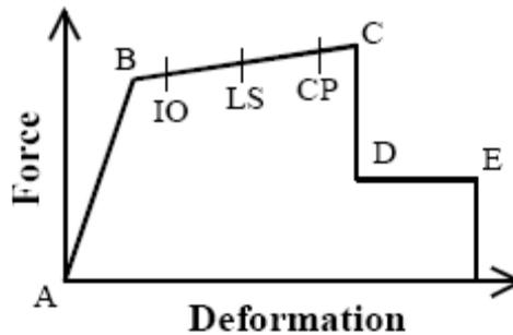
Figure 9. Force-deformation relation for hinges (reprinted from public domain document FEMA 356, the precursor to ASCE/SEI 41-06) showing the definition of acceptance criteria and performance states
