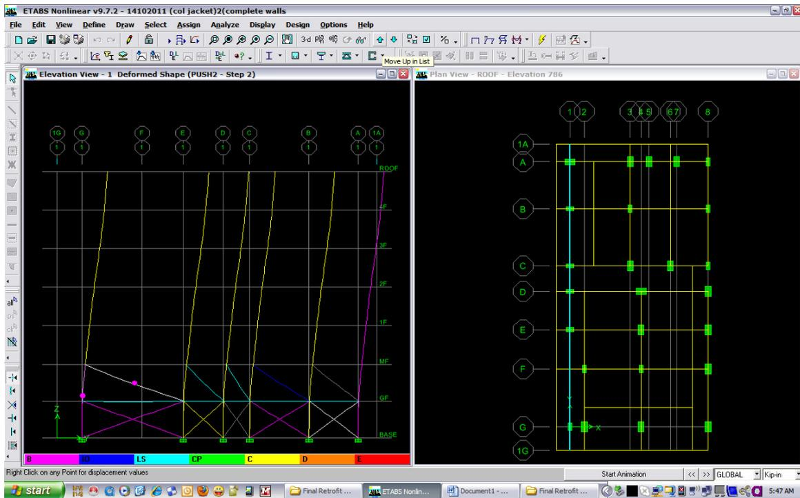
Mechanism or Deformed shapes at Performance Point - grid-1
