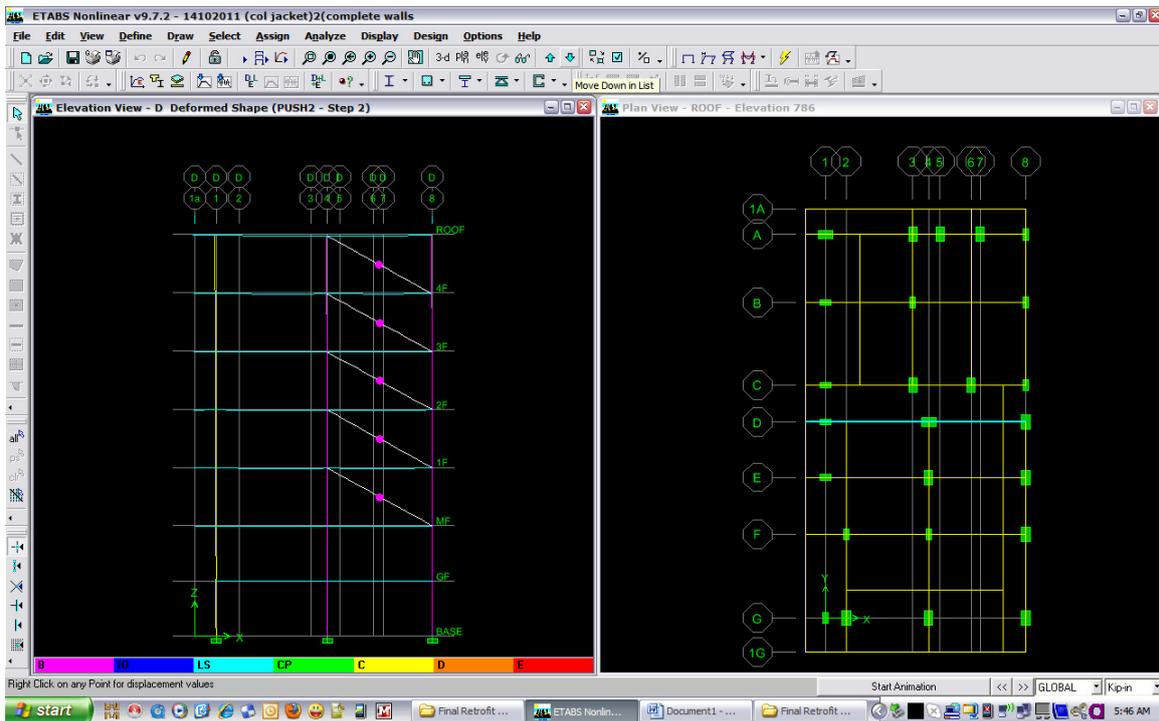
Mechanism or Deformed shapes at Performance Point - grid-D
