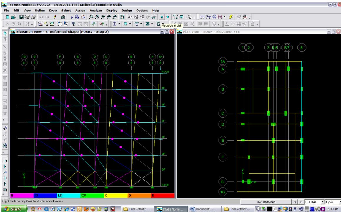
Mechanism or Deformed shapes at Performance Point - grid-8
