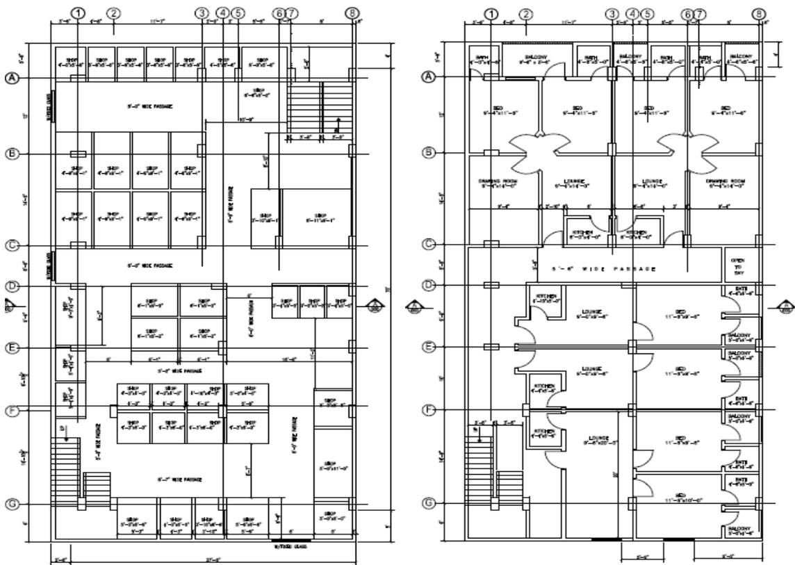
Figure 3. Architectural layout of mezzanine floor (left) and typical upper floors (right)
