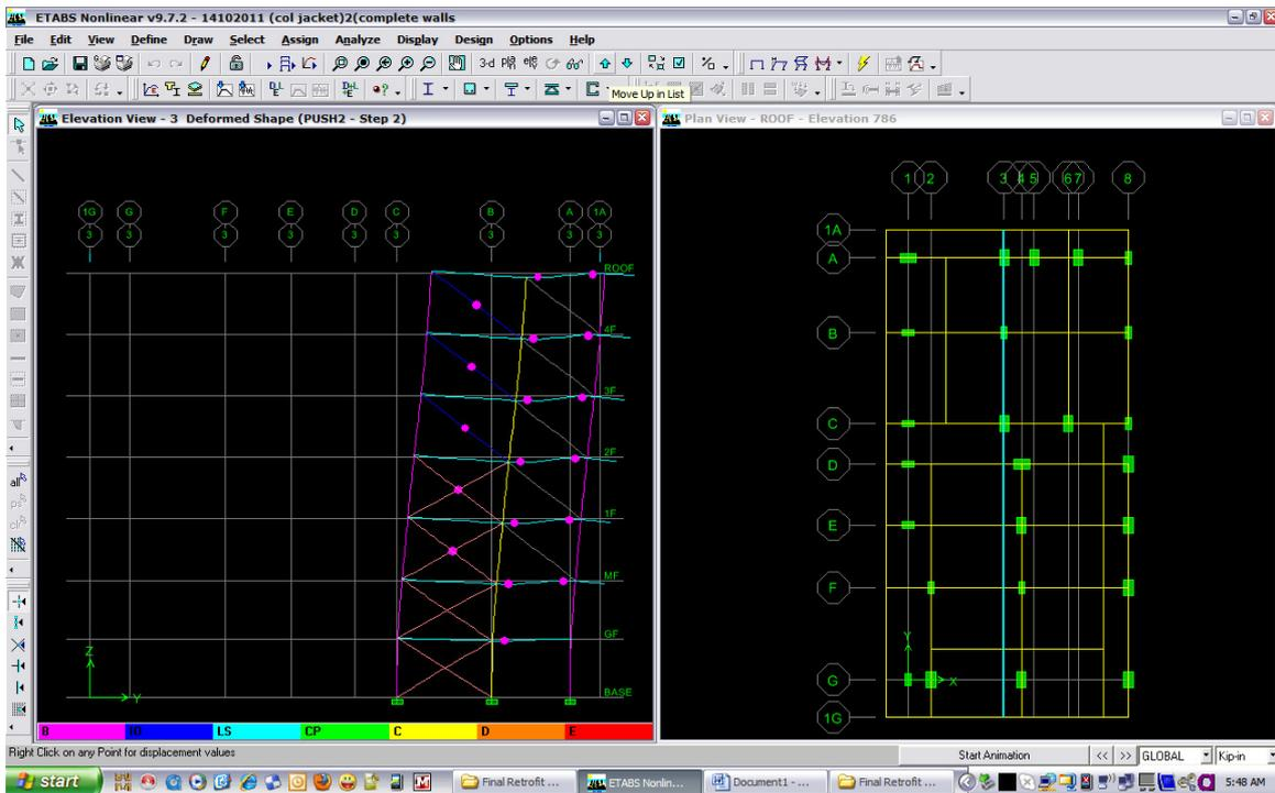
Mechanism or Deformed shapes at Performance Point - grid-3
