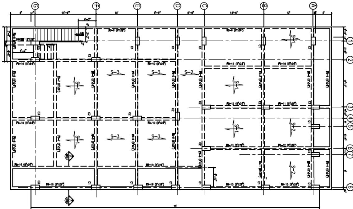
Figure 7. Structural layout of typical upper floors
