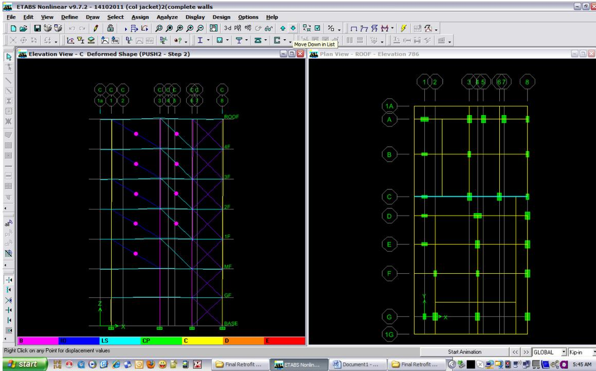
Mechanism or Deformed shapes at Performance Point - grid-C
