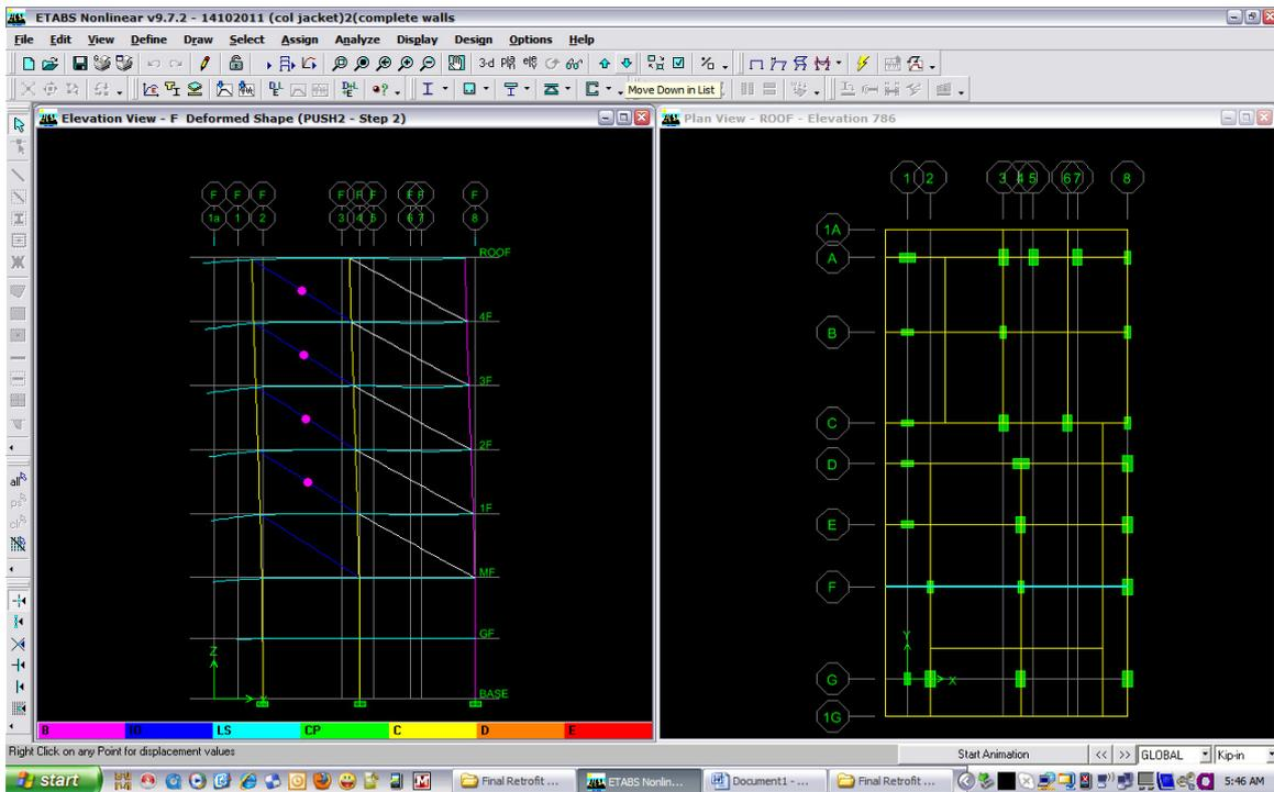
Mechanism or Deformed shapes at Performance Point - grid-F
