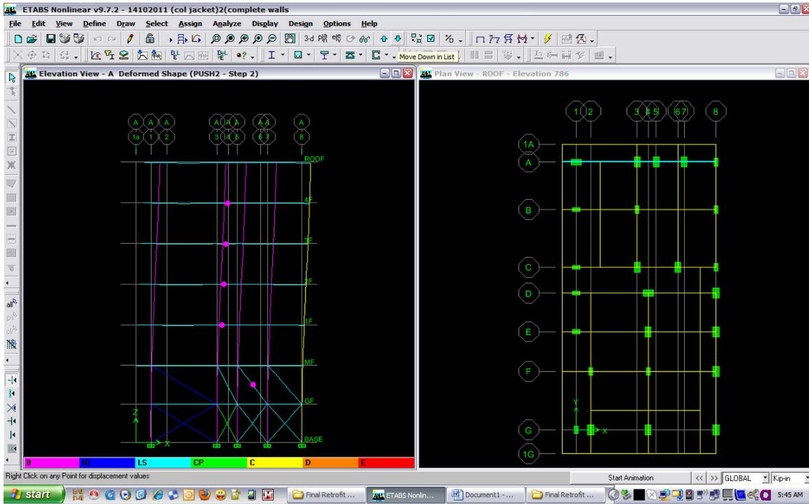
Mechanism or Deformed shapes at Performance Point - grid-A
