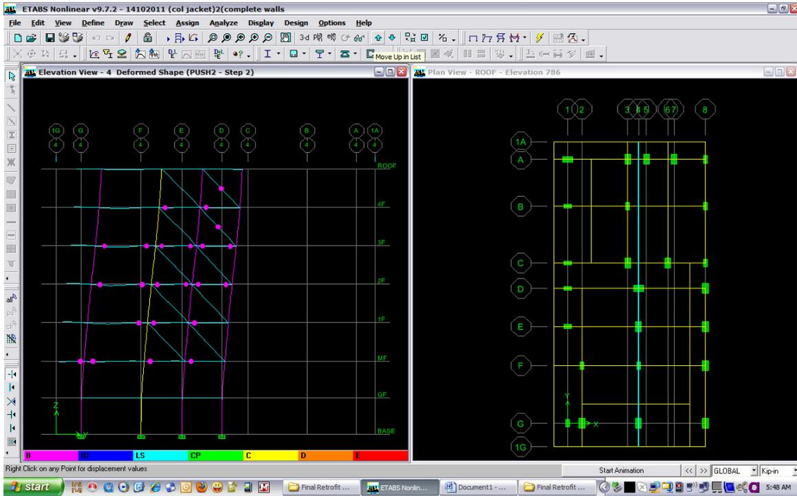
Mechanism or Deformed shapes at Performance Point - grid-4
