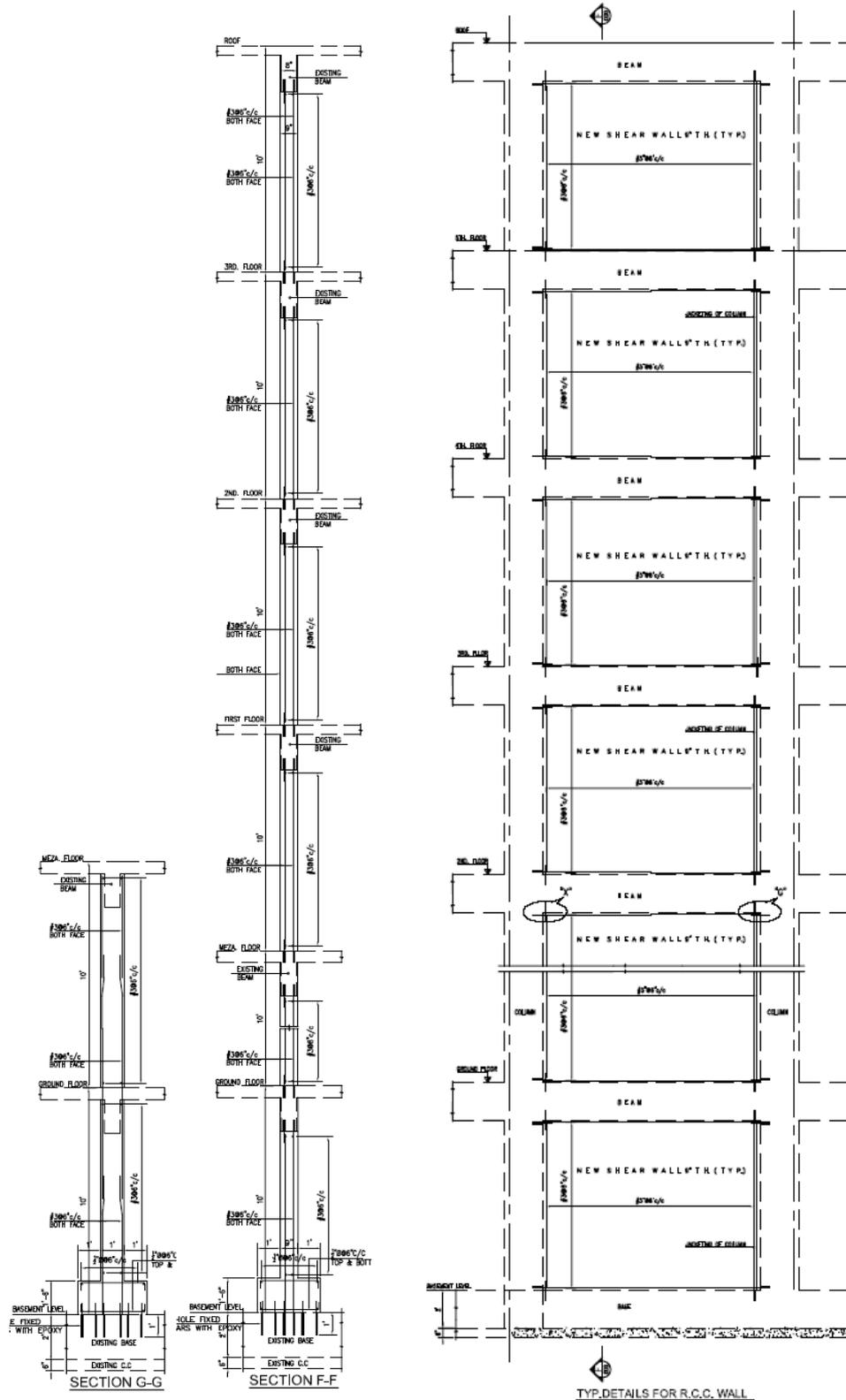
Figure 16. Proposed retrofitting details for new RCC shear walls
