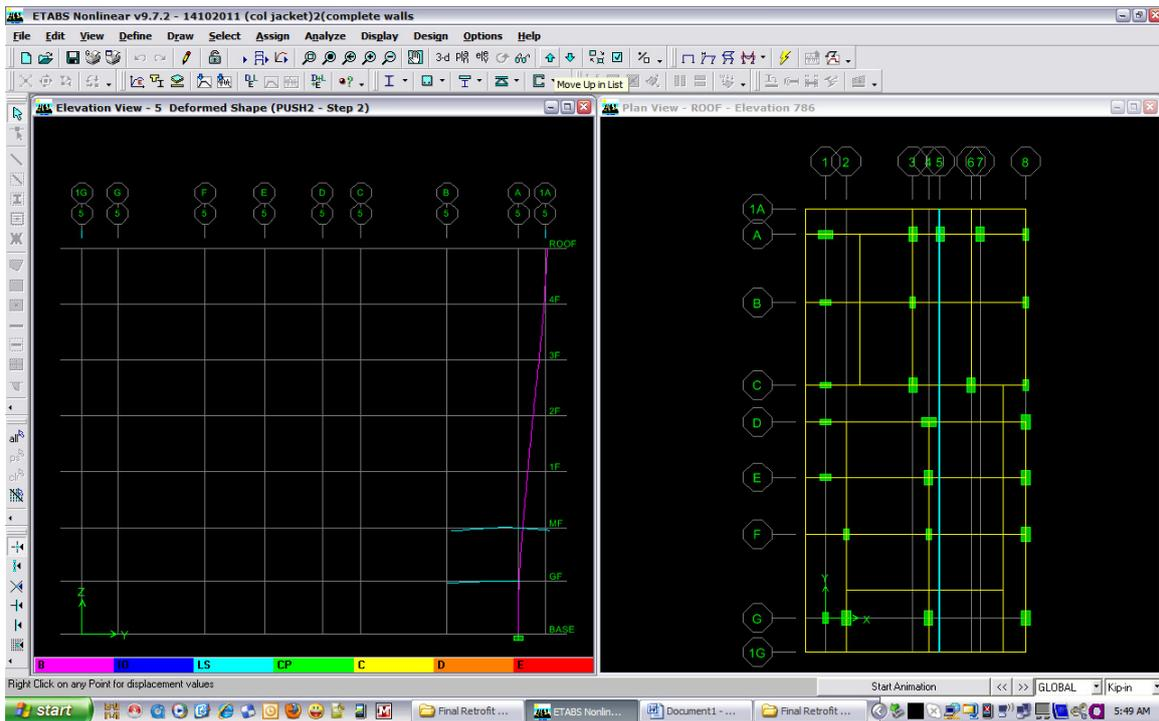
Mechanism or Deformed shapes at Performance Point - grid-5
