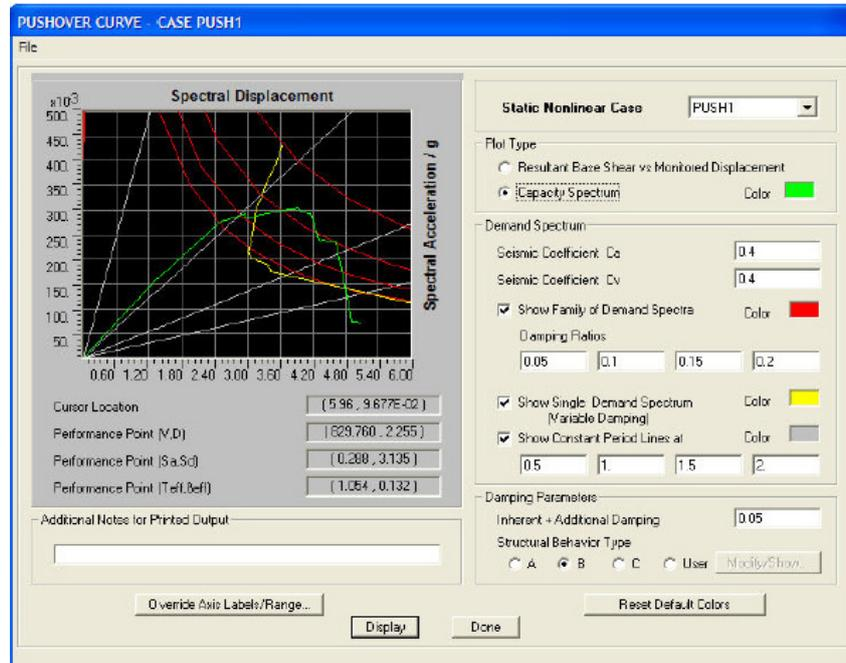
Figure 11. Performance level for seismic forces in X-direction
