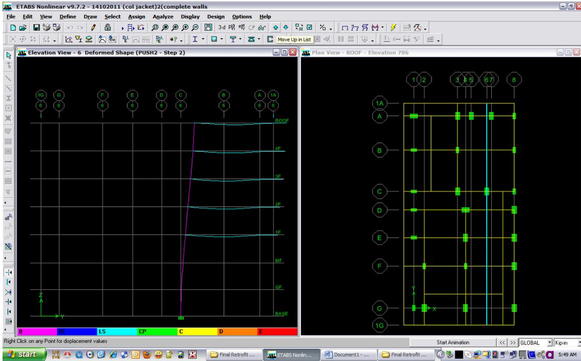
Mechanism or Deformed shapes at Performance Point - grid-6
