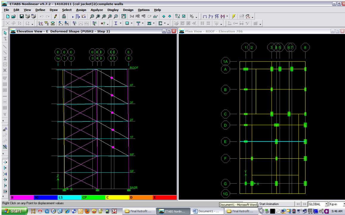
Mechanism or Deformed shapes at Performance Point - grid-E
