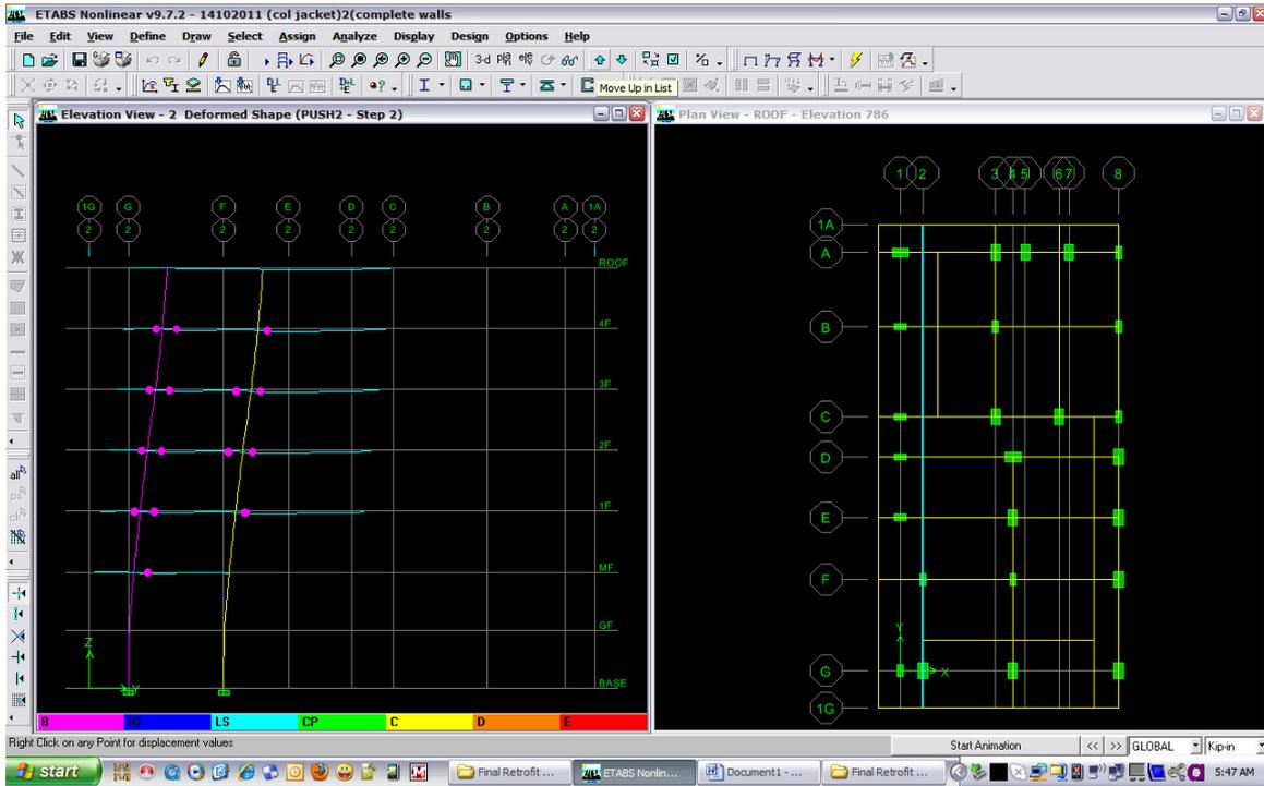
Mechanism or Deformed shapes at Performance Point - grid-2
