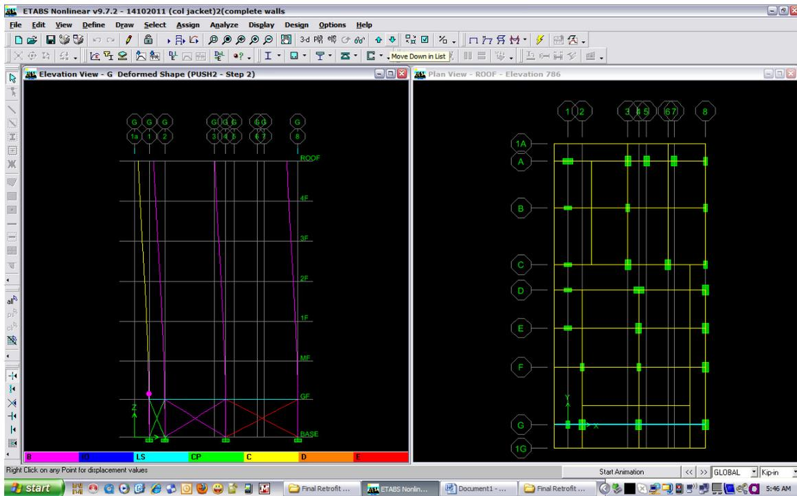
Mechanism or Deformed shapes at Performance Point - grid-G
